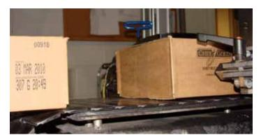
The Videojet 2300 Series printer recycles ink used for automatic printhead maintenance and uses it for printing after filtration. Robinson appreciates that the ink is not wasted and estimates that Golden State Foods can print on thousands of boxes from each can of ink. Plus, the cans are easy to install, and all of the Videojet printers at Golden State Foods require the same type of ink, eliminating the possibility of installing the wrong type of fluid in a printer.
